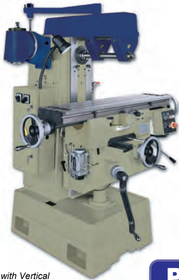
PBM-UM1 with Vertical Head on Swivel Arm (Pictured without Guarding and Splash Tray)
